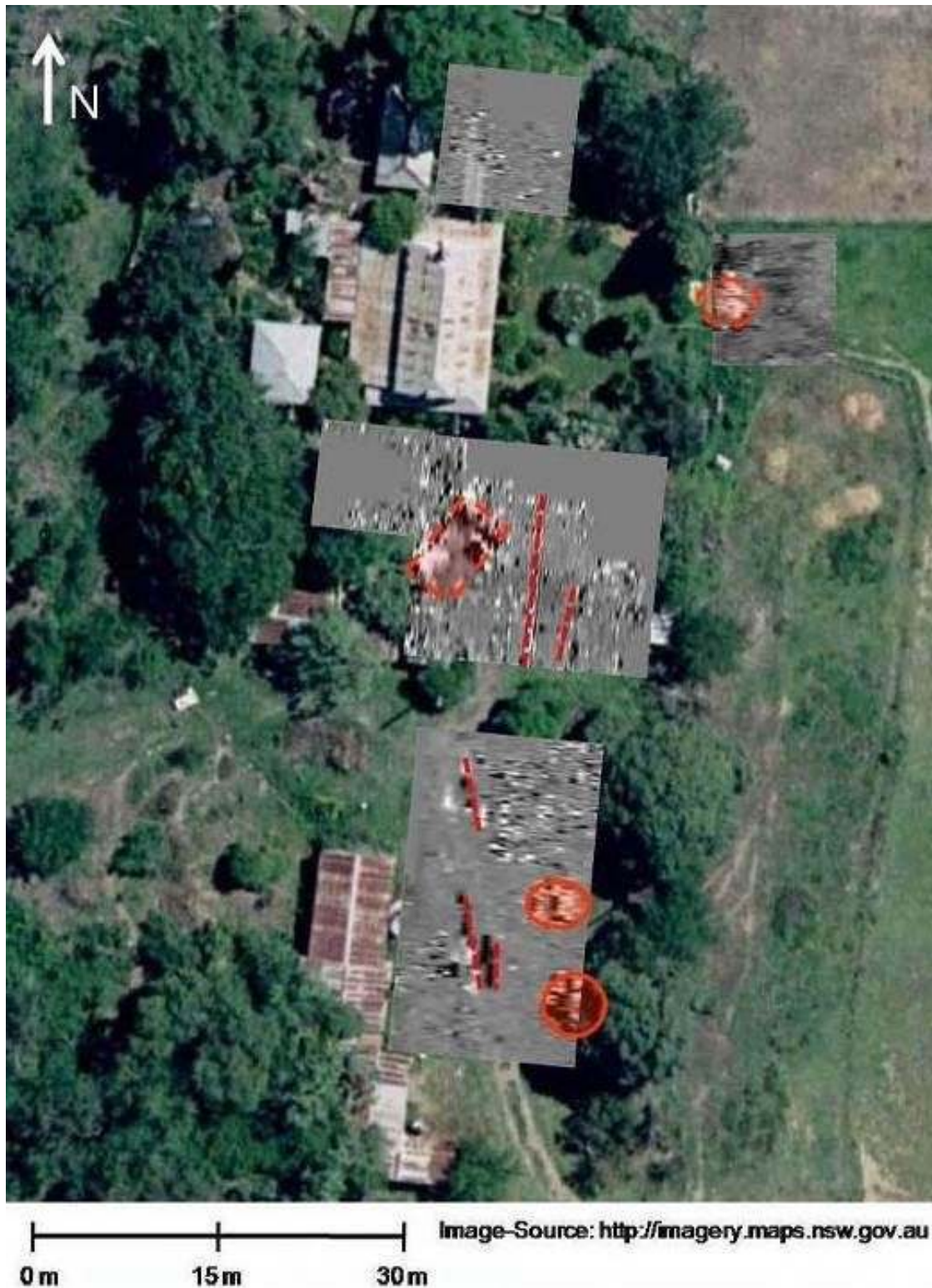
Figure 80. Ground penetrating radar image showing the location of a former structure (dashed rectangle), possibly the remains of the former cream shed (previously located closer to the road), underground silos (circles) and services (dashed lines). Source: GML CMP 2013, Archaeological Computing Laboratory, University of Sydney, 2008.
